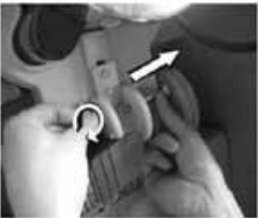
Step 4 - Unload control handle and install screw.
